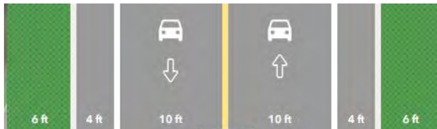
Figure 4: 1st Street, Section near Union St
